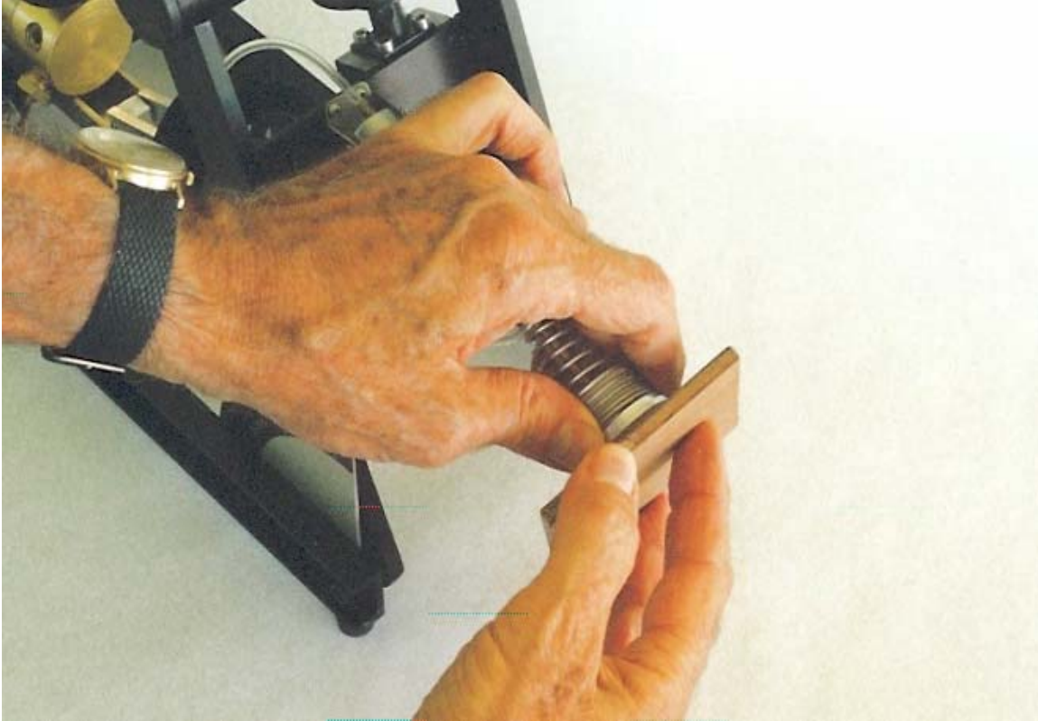
Figure 4. Grip the testfoot firmly with one hand while sanding with the other in a circular motion.
