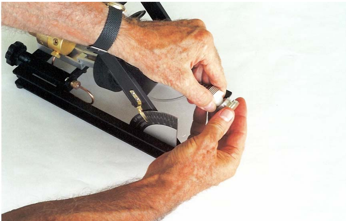
Figure 2. Slide the spring back and grip the plastic nut securely when changing testfeet. Be sure not to release the spring until the replacement foot has been screwed in. Be careful not to cross-thread it so as to damage the nylon threads.
